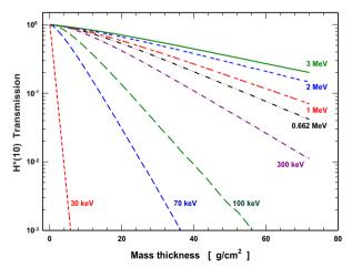
Figure 6. Ambient dose equivalent transmission in cantera.
