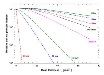
Figure 4. Collided photon transmission in cantera.
