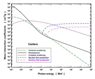
Figure 1. Photon mass interaction coefficients in cantera.
