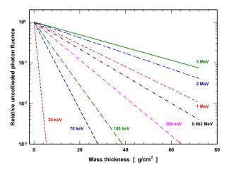
Figure 3. Uncollided photon transmission in cantera.
