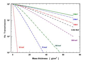
Figure 5. Kerma in air transmission in cantera.
