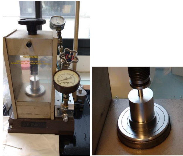
Figure 2.10. Manual hydraulic press and pressing die during the making of green ceramics.
