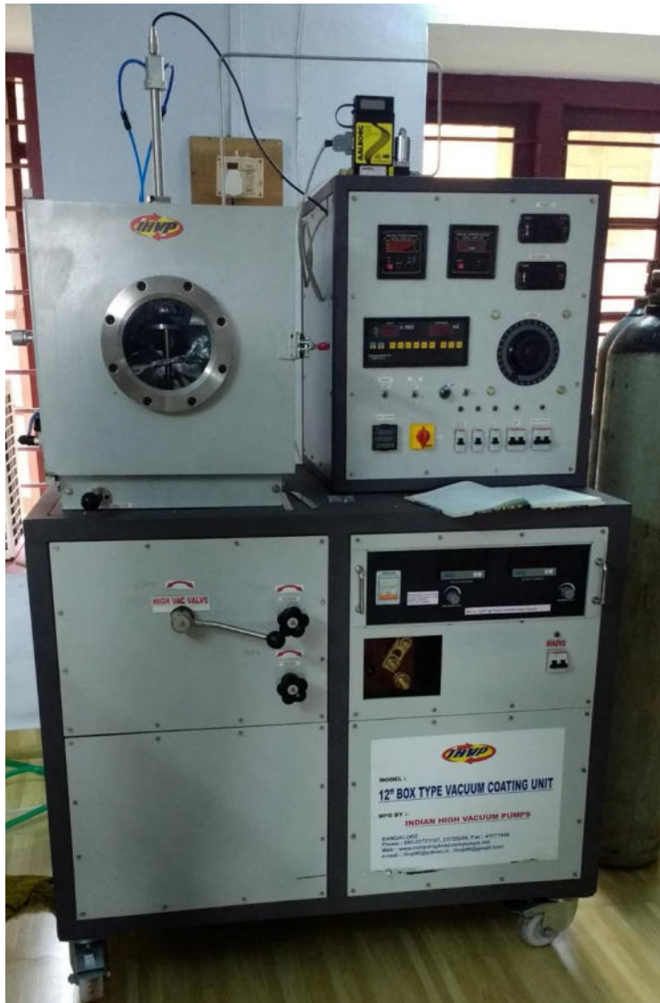
Figure 6.5: Vacuum thermal evaporation unit used for the deposition of the nanorods.
