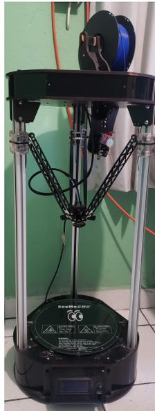
FIGURA 6.1: Impresora 3D Rostock Max V2
