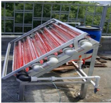
Fig. 13. Photocatalytic Solar CPC Reactor, UANL.
