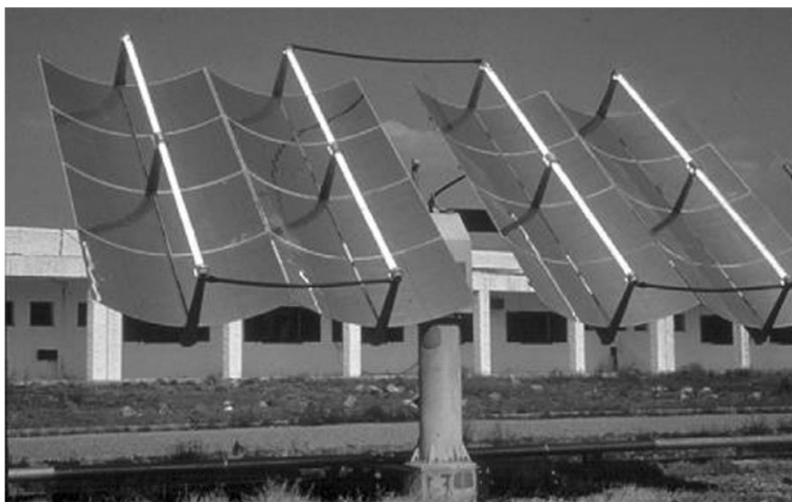
Figure. 4. Parabolic trough photocatalytic reactor at Plataforma solar de Almeria (Spain) (Malato et al., 2007).
