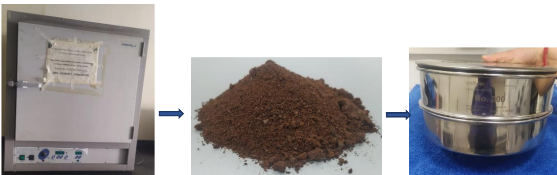
Figure 19. Spent coffee grounds dried at 100 °C, sieved through mesh No.200
