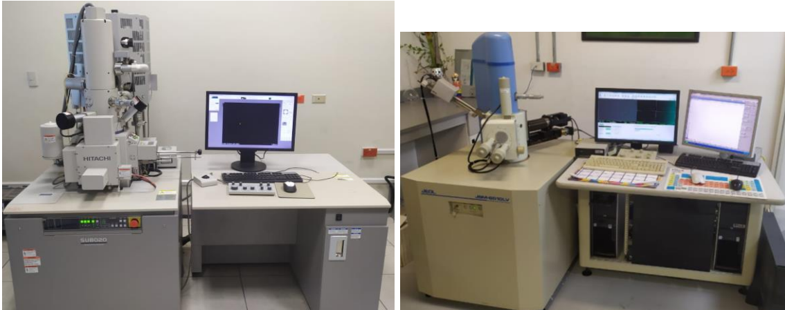
Figure 24. Field emission scanning electron microscopy a) Hitachi, model SU8020. b) JEOL, model JSM- 6510LV
