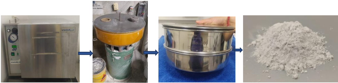
Figure 18. Dried at 60 °C, Volcanic sand was ground in a ball mill, VA sieved through mesh No.200
