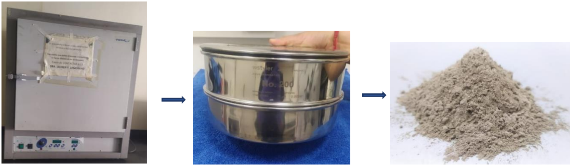
Figure 15. Dried at 60 °C, OPC sieved through mesh No.200
