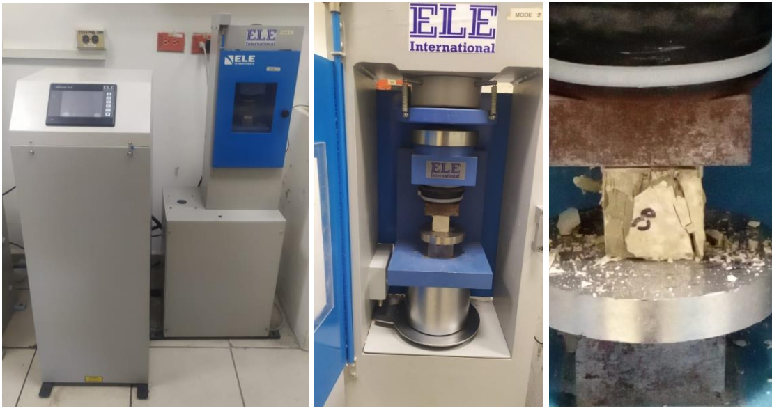
Figure 21. Compression testing machine ELE International
