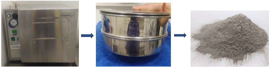
Figure 17. Dried at 60 °C, FA sieved through mesh No.200
