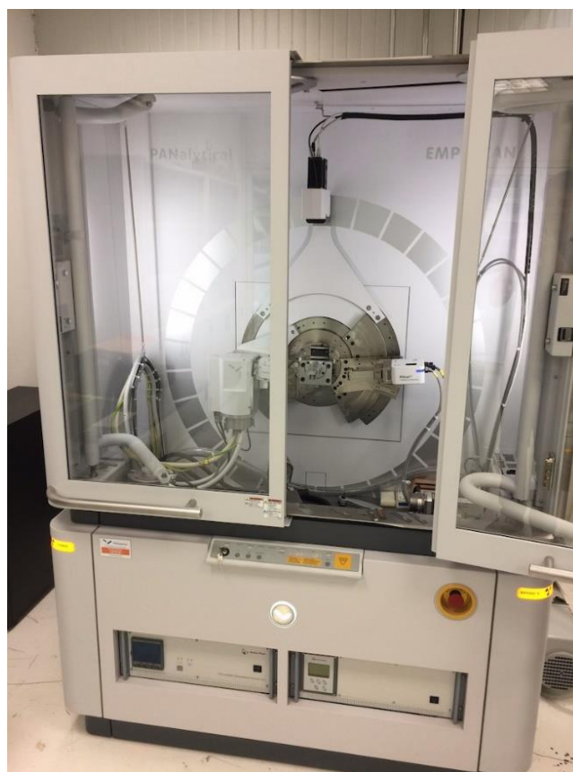
Figure 23. Empyrean Panalytical X-Ray Diffractometer
