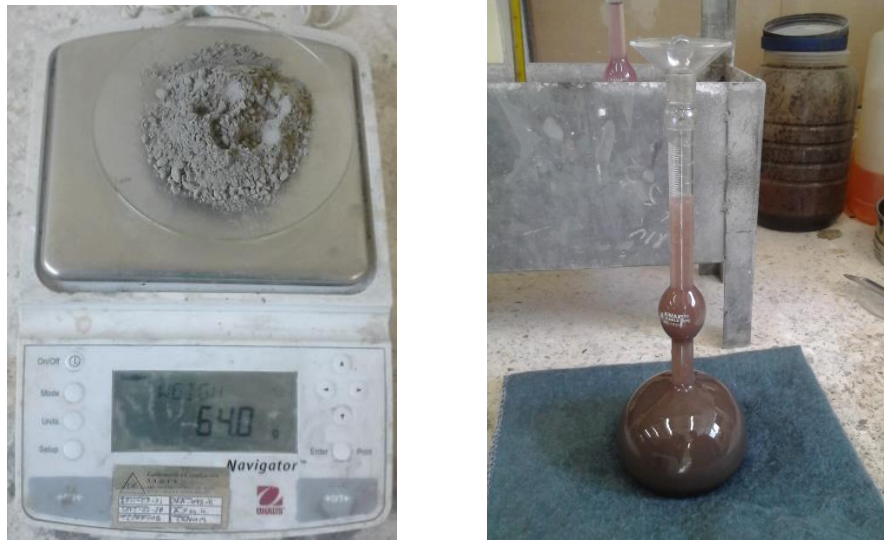
Figure 26. The density of Portland cement using the Le Chatlier apparatus
