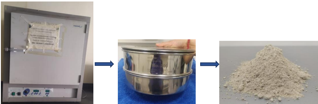
Figure 16. Dried at 60 °C, CSA sieved through mesh No.200
