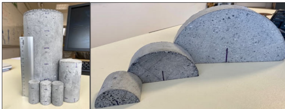
Figure 45. Notch of the Mortar samples cut in half circle.
