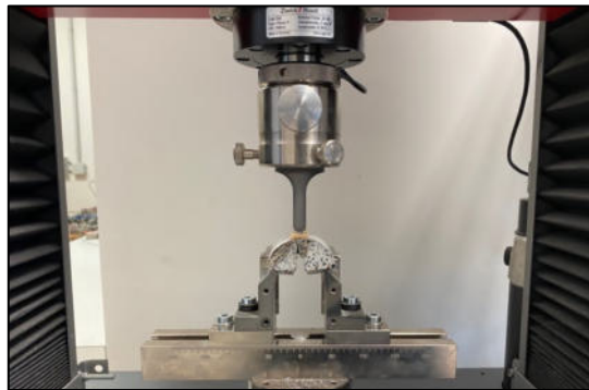
Figure 50. Mortar sample of 5 cm of diameter
