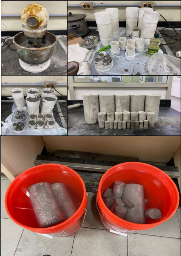
Figure 44. Preparation of mortar specimens
