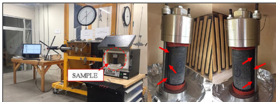
Figure 67. Set-up for high temperature tests in limestone samples. The arrows indicate the location of through cracks after the test at 100° C.
