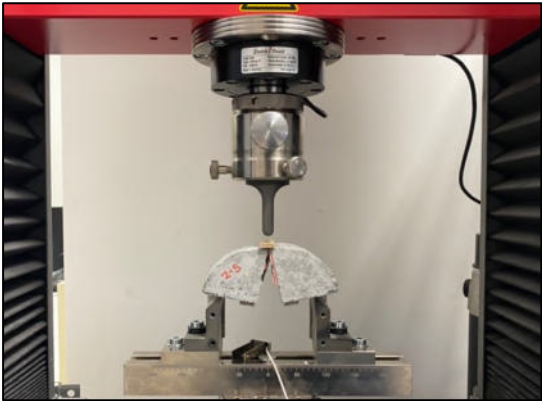
Figure 49. Mortar sample of 10 cm of diameter
