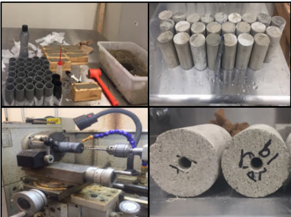
Figure 34. Preparation of synthetic rock specimens
