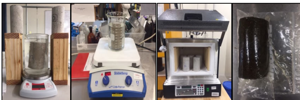
Figure 35. Drying and open porosity test on synthetic and limestone specimens
