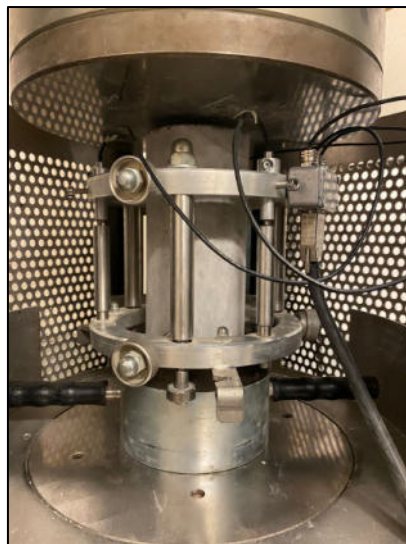
Figure 51. Mortar specimen during the test to calculate the young modulus.
