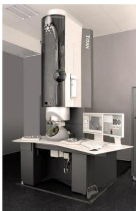
**Figura 9.** Microscopio TEM marca FEI, model Titan G2 80-300. (Imagen recuperada de: [https://www.researchgate.net/figure/FEI-Titan-80-300-transmission-electron-microscope-photograph-by-courtesy-of-Ralf-Uwe\\_fig1\\_292343701](https://www.researchgate.net/figure/FEI-Titan-80-300-transmission-electron-microscope-photograph-by-courtesy-of-Ralf-Uwe_fig1_292343701))
