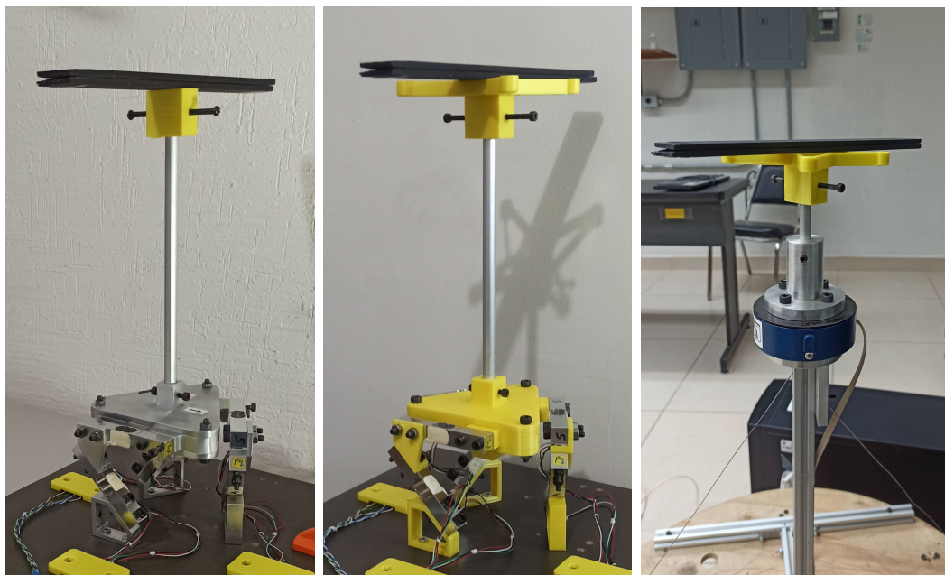
(a) Al-6061 testing bench (b) PLA testing bench (c) JR3 force-torque sensor
