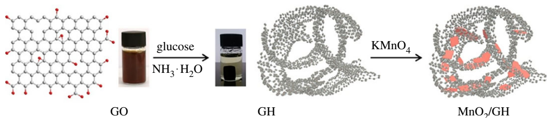
Figure 28. Schematics of the synthesis process of GH and MnO 2 /GH. Adapted from ACS Publications.
