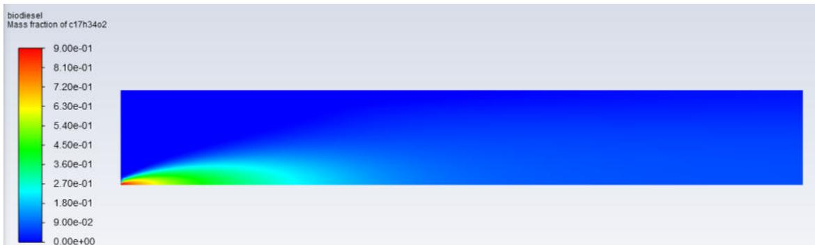
**Figure 21.** Biodiesel mass fraction profile for 0.9 biodiesel + 0.1 Levulinate mixture with adjusted air:fuel ratio
