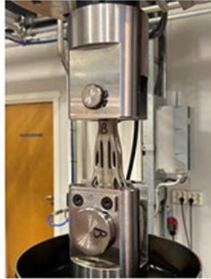
Figure 4.4 Connecting rod fatigue test bench[36].
