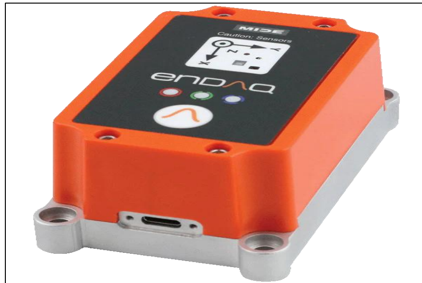
Figure 14. enDAQ W8-D40 sensor
