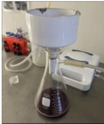
Image 1: Solid: liquid extraction technique for the preparation of wine pomace extract
