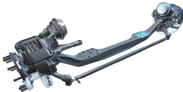
Figure 2.3.3 Non-driving front axle with wheel end assembly [22].
