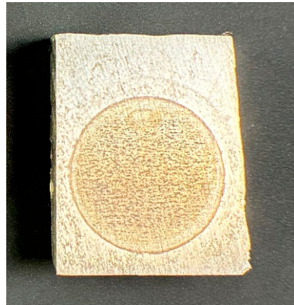
Figure 1. AA2024 verification specimen with a known corrosion area of 143.158 mm 2 corresponding to the circular corroded region.
