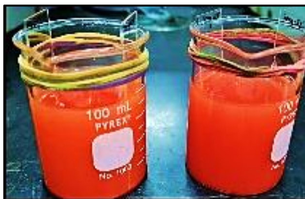
Figure 2.1. Schematic diagram of chemical bath deposition method under ambient condition.
