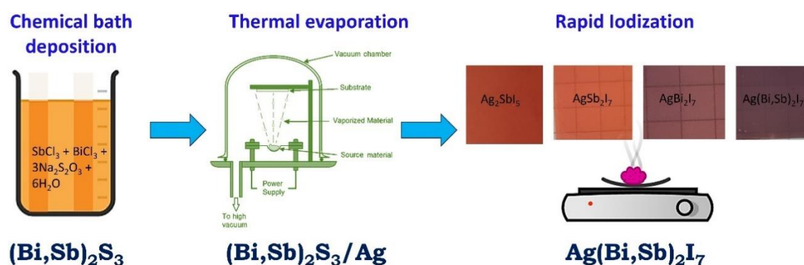
Figure 5.1. schematic diagram of mixed alloy rudorffite \text{Ag}(\text{Bi,Sb})_2\text{I}_7 thin film synthesis.
