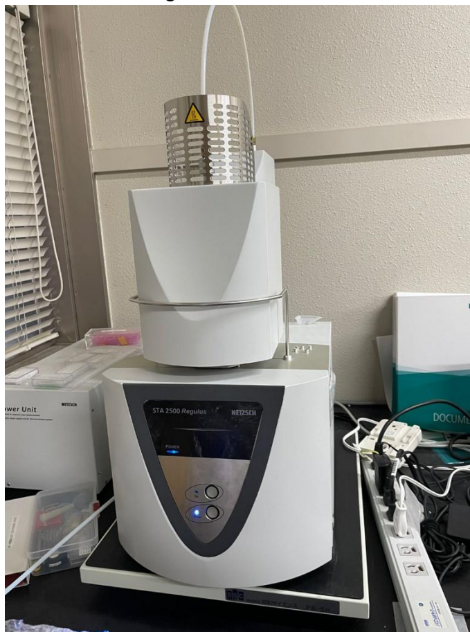
Figure 3. NETZSCH STA 2500 Regulus simultaneous thermal analyzer used for the thermal characterization of \text{HfO}_2 nanoparticles. Thermogravimetric analysis (TGA) and differential scanning calorimetry (DSC) measurements were performed to evaluate mass loss behavior.
